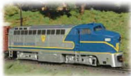
DCC ON BOARD™ locomotives feature dual-mode digital command control decoders enabling operation with a standard DC analog power pack or any NMRA-compliant Digital Command Control system. Speed, direction, and lighting control.
