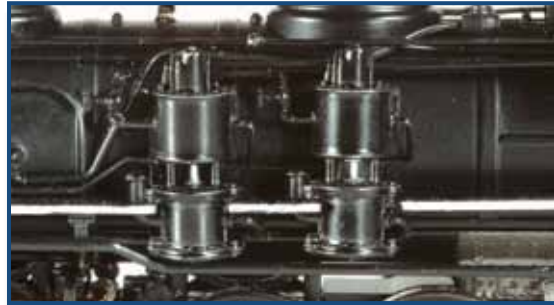
Below: Details such as these dual 11" single-stage compressors accentuate the unique appliances of each prototype.
