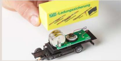
**Trunks and tarpaulins 6.8 m long in the original:** Intermediate plate of conversion chassis can be shortened. In the first picture this is approx. the rear length of the black intermediate plate, which is longer than the green PCB.
