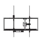
Comprised of a track-bound gantry crane transversally handling unit load devices along the transshipment tracks, dead-end sidings and extensive storage areas as well as a gantry-like crane jib with control cabin, trolley and telescopic grappler spreader that, like lifting slings, seizes the loads to be transshipped, such as e.g. containers and interchangeable bodies, and places them in the targeted position. Suitable for the representation of handling
