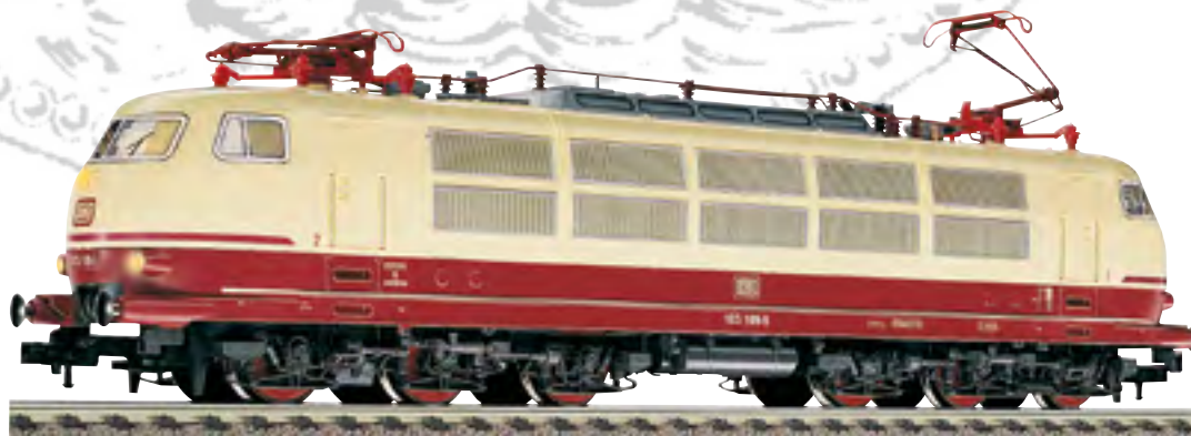
437601 Electric locomotive BR 103.1 of the DB, Epoch IV with digital interface
