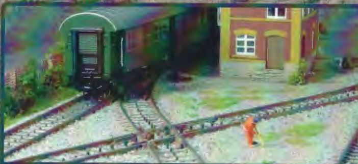
In the scene with the interlocking block you see the double-slip switches.
