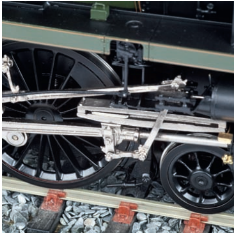
Uniquely, the valve gear is designed to be reversible, as on full-size steam locomotives.
