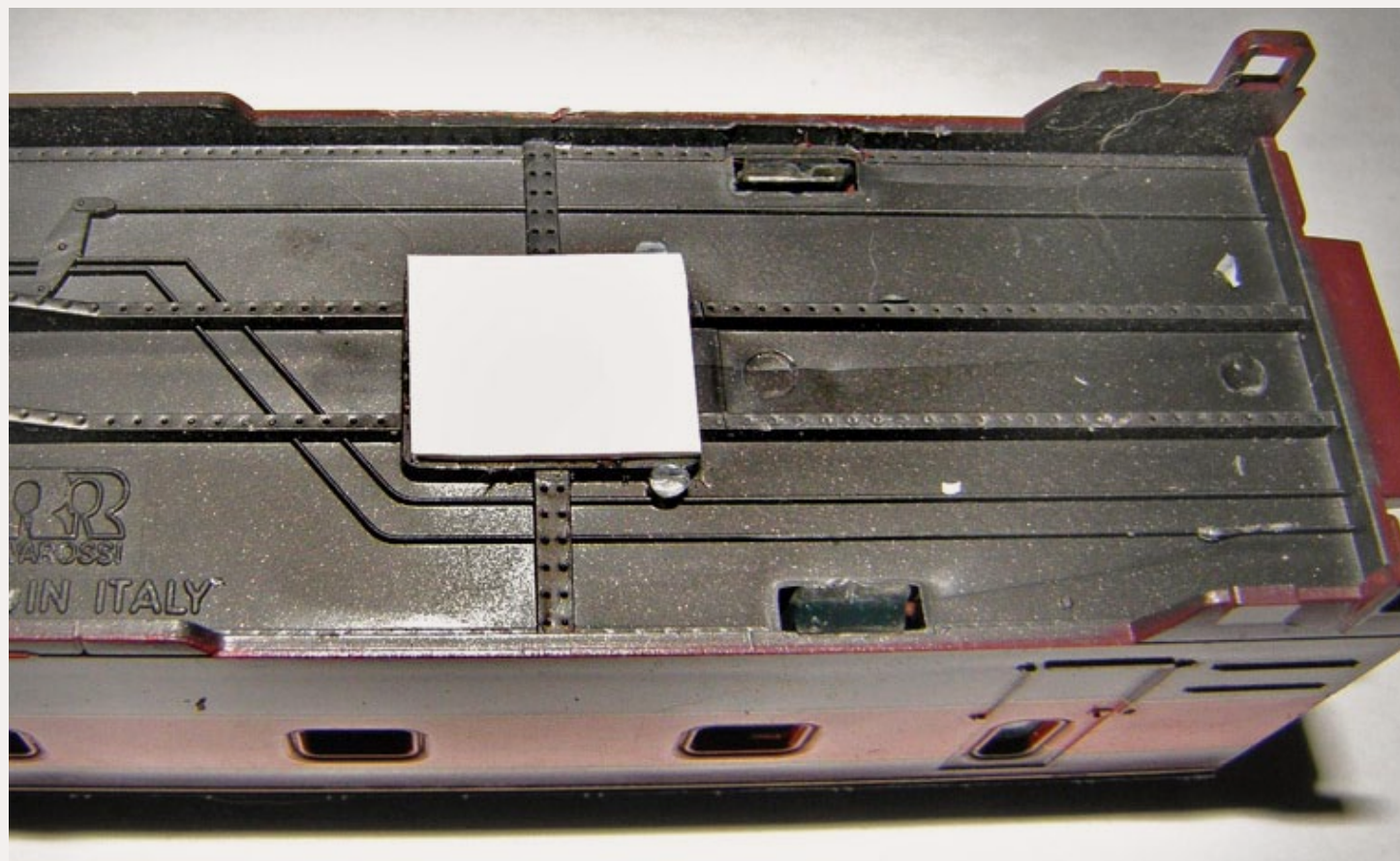
Figure 6: Using A.C.C. I cement a piece of .030 styrene cut to the size of the pad over the old pad to build up the clearance which existed with the old bolster. This is not as tall as the old bolster which will yield a more prototypic space between the truck and the underframe. It will also eliminate much of the wobble normally associated with Rivarossi passenger cars. File edges of the new pad to conform to the shape of the old pad and slightly round the edge for a nice finish.
