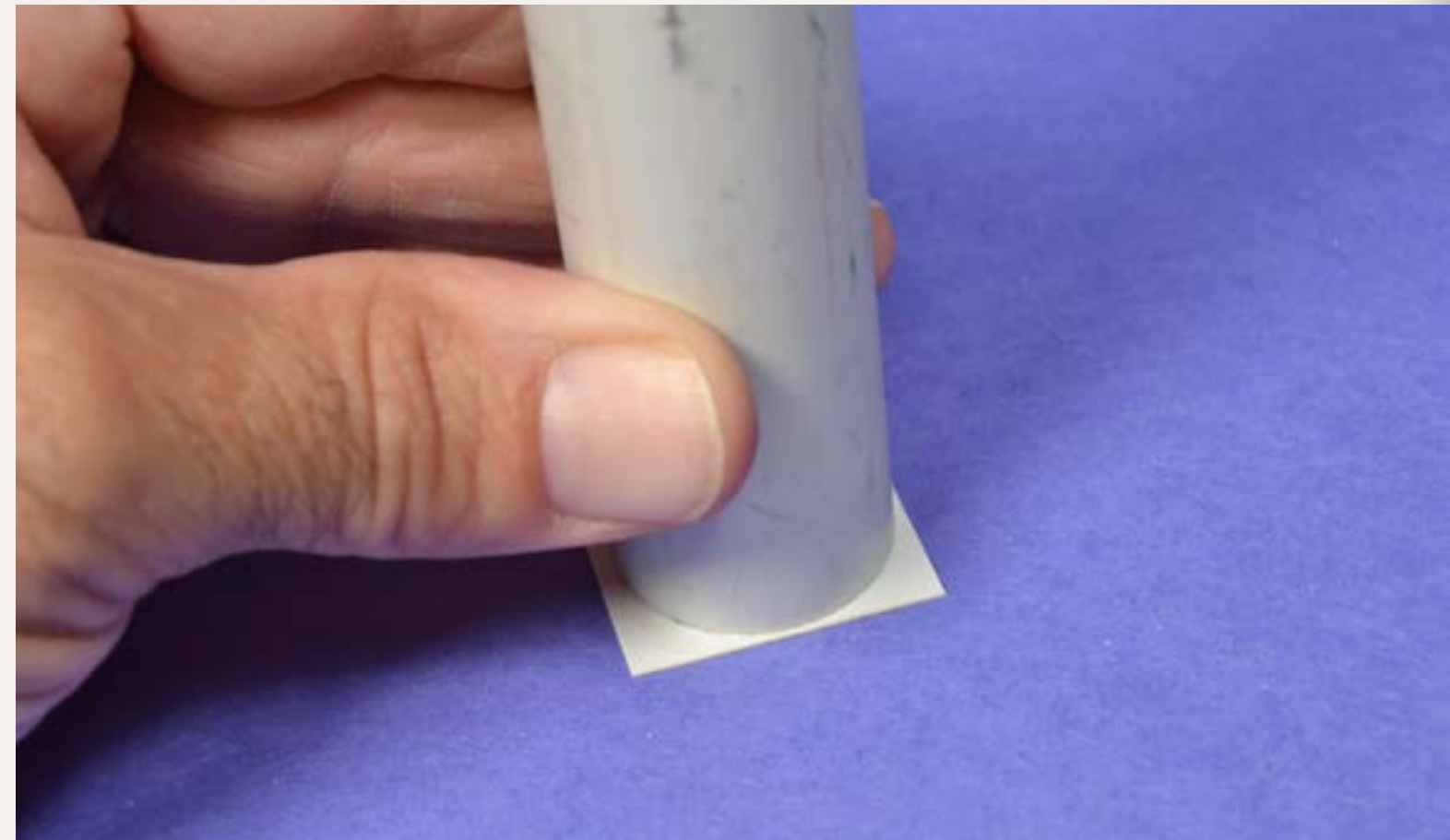
Figure 3: Glue the styrene to the ends of the PVC pipe using gap-filling cyanoacrylate glue.
