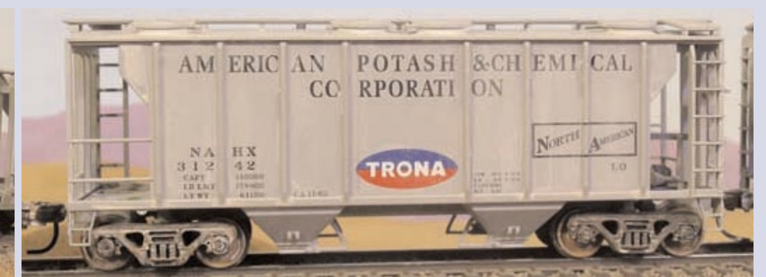
Figure 8 (All 4 cars): Loading potash is a dusty business. It settles on all parts of the car including the trucks. With rain and weather on the road, streaks form on the sides and seal potash coating of the white chemical to the car. I use a wash of flat white latex indoor house paint, mixed with a little alcohol to give this effect. A flat edged brush can be used to pull white streaks down the car side.
