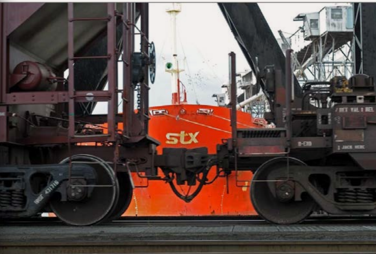
Figure 2: Railroad car wheels are sized according to the weight of the freight car and can range from 28 to 38 inches for cars in general service. Photo by Graham Line.
