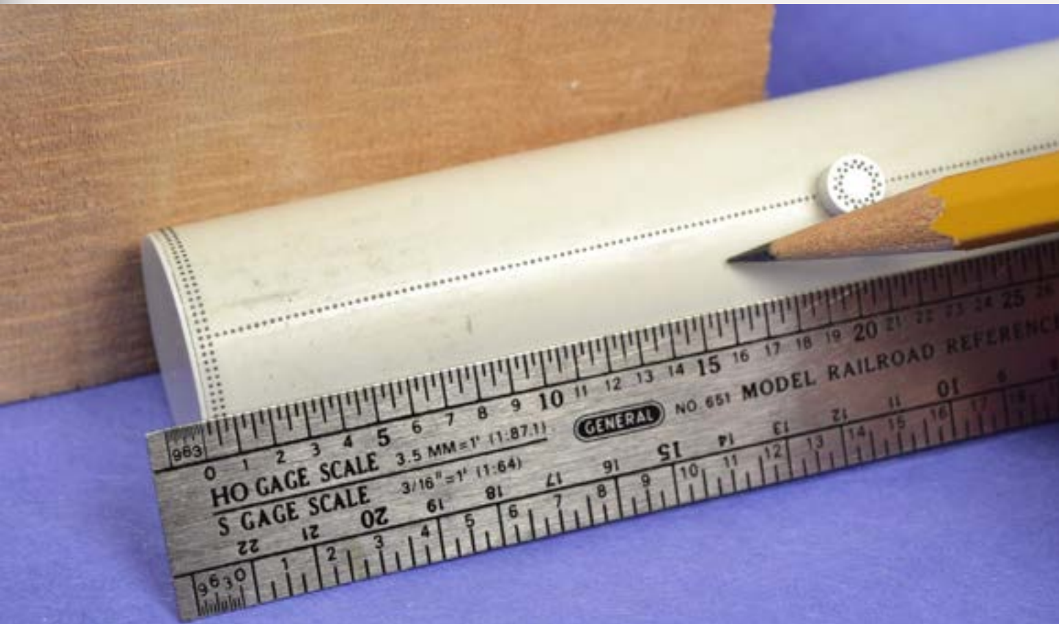
Figure 8: Mark 8' increments along each side of the top of the tank and near the bottom. Use these marks to line up the single rows of vertical rivets.
