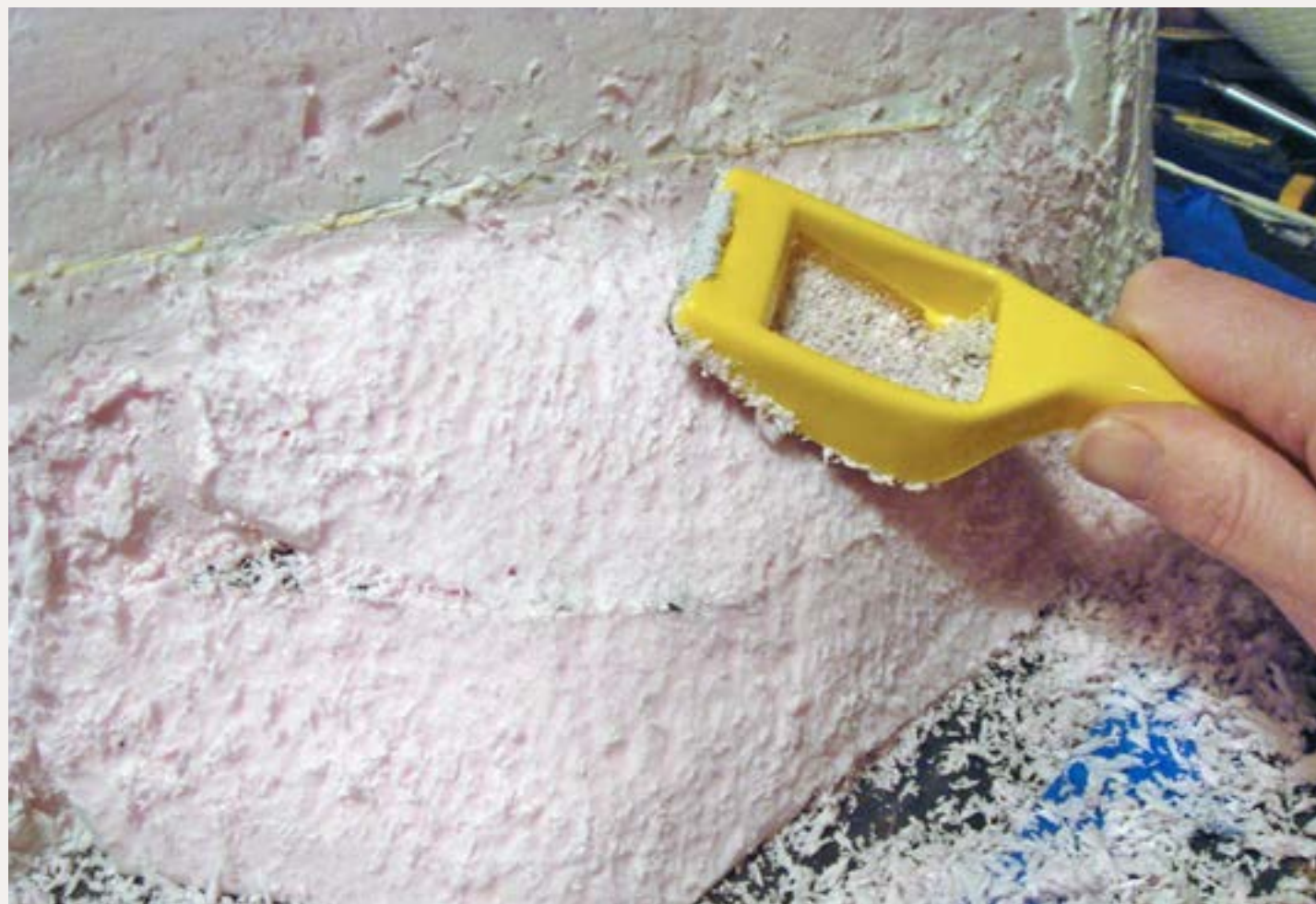
Figure 6: Kids can shape foam into hills with a forming tool, the model railroader's version of the "safety razor." Any foam work should be done with a mask and with a shop vac close at hand (a great job in itself for a youngster).
