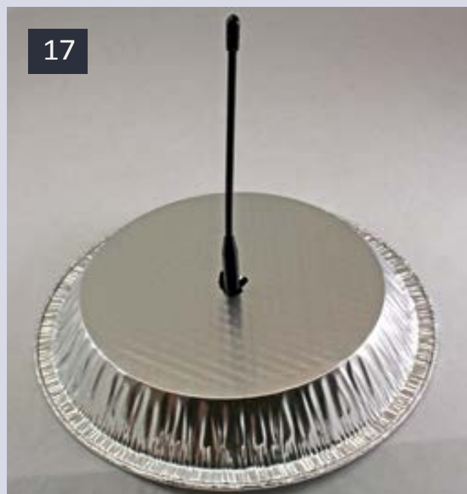
17: NCE RB02 with a pie pan ground plane.
