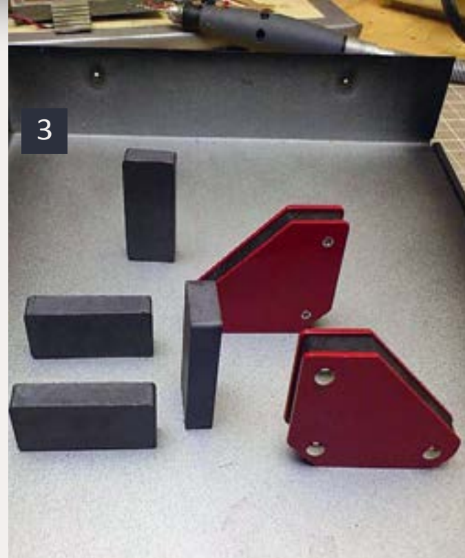
3: Kevin Rowbotham used a discarded sheet metal electronics chassis, and magnets sold to welders, to create his magnetic gluing jig for structures and car kits. (Kevin Rowbotham photo).
