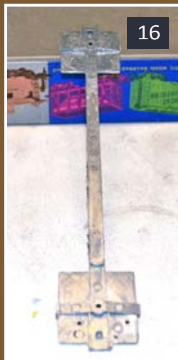
14-17: Burrs removed and chassis painted black.
