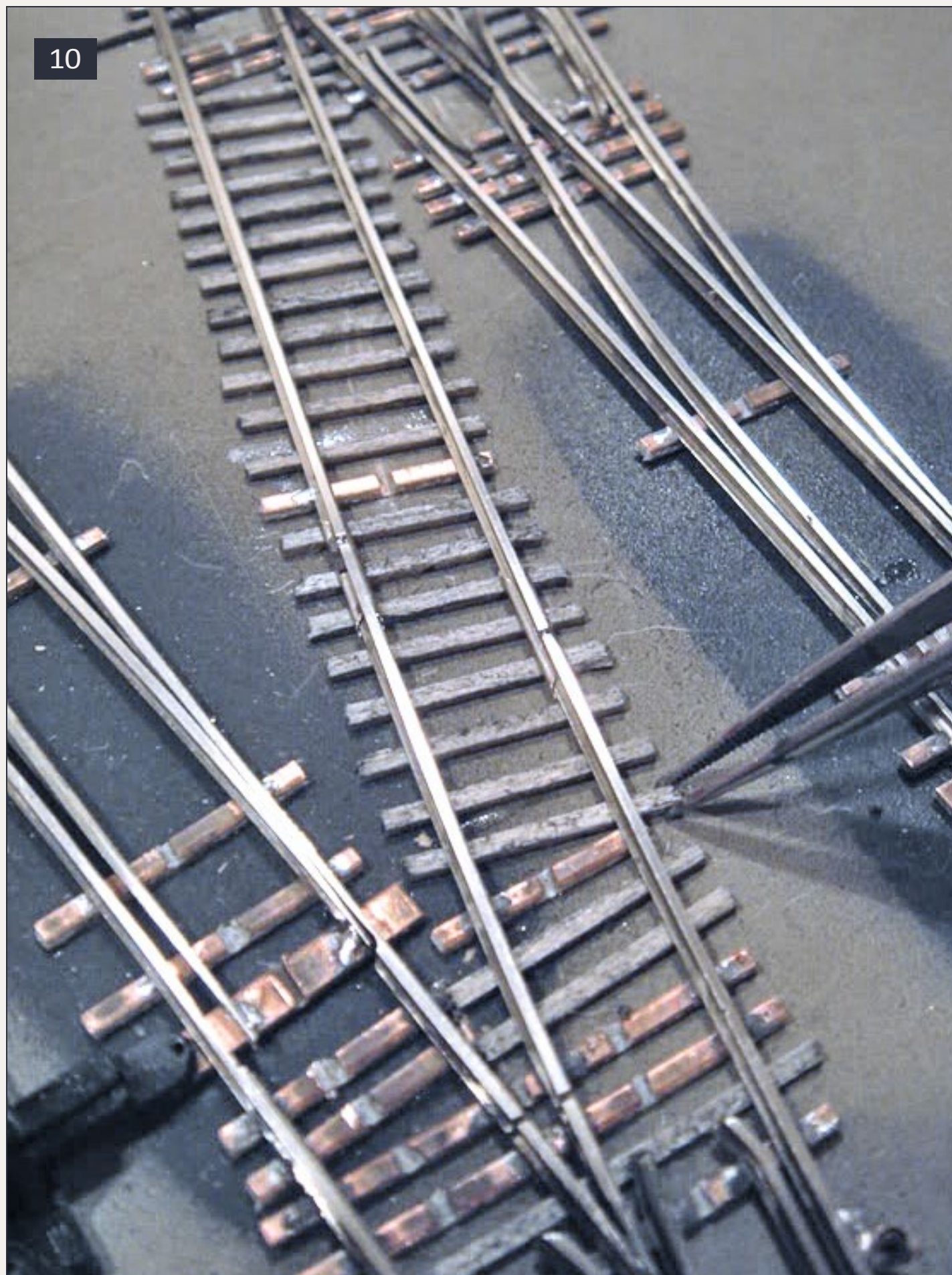
10: Filling in the gaps in the ties with replacement ties made from stained 1/32" x 3/64" basswood strips. I just coat the back of the tie with white glue and slip it in place using tweezers.
