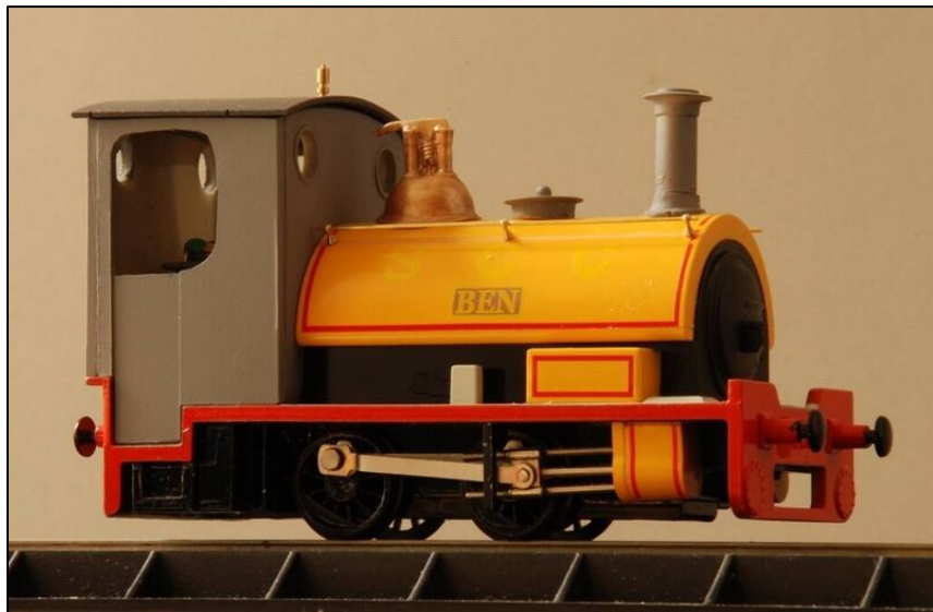
"Poppy". Smallbrook Studio's kit to convert a Bachmann Thomas & Friends "Bill" or "Ben" into a good representation of a 5.5mm scale Peckett. ( Photo: Smallbrook Studio)
