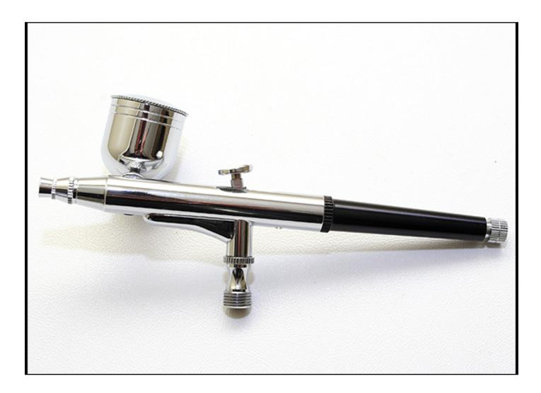
The internal mix brush is the most controllable of the two types, and will allow you to paint finer detail with greater control. As most of these brushes have a two stage control over both the air pressure and paint flow, combined with the internal mix means that finer lines can be achieved. The air is controlled by depressing the button and the paint by pulling the same button backwards, thus increasing the paint flow.
