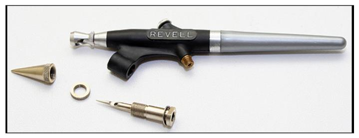
The air pressure builds up as you depress the trigger it causes more paint to be sucked up into the nozzle, and to be mixed into the jet of air giving the spray.
