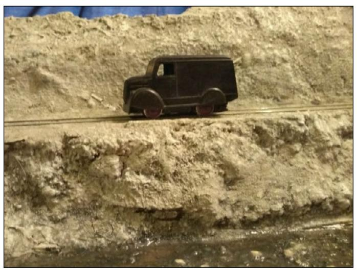
The un-numbered Trojan van is a Dinky die cast model powered by a Bachmann OO DMU chassis, it's not a particularly good runner though so it might get a permanently coupled trailer to provide additional electrical pick up.
