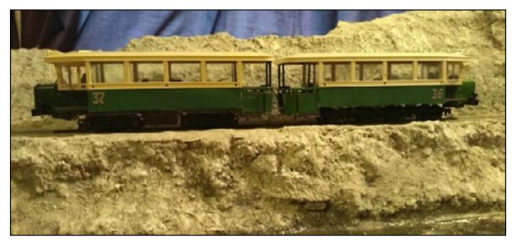
Railcars 36 and 37 are a matching pair of Renault buses by Solido, one on an Athearn HO diesel chassis, the other on a pair of OO coach bogies. These were built for On30 scale and are pretty big if used on the modules though not excessive for rail rather than road carriages.
