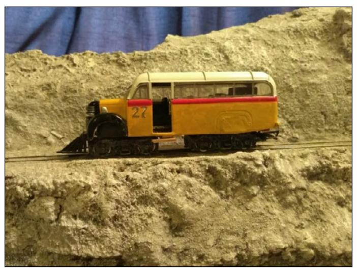
27 is a model of a Maltese bus riding on a shortened Bachmann F7 mechanism. In common with most of the railcars its rear wheel arches have been "plated over". In this case I used filler but it can be simpler, and more durable, using card or tinplate sheet to do the job.
