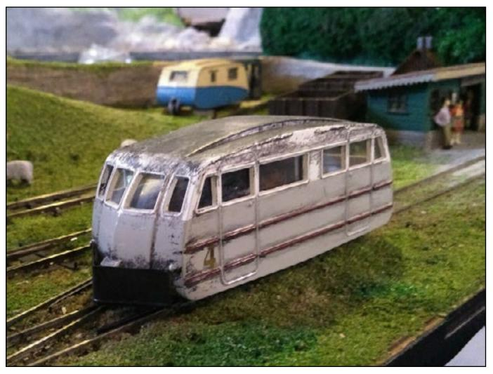
Railcar number 4 is an oddity. If it looks vaguely French that's because it is, it's a Dinky model of a French caravan with has two doors on each side, much more in keeping with a rail vehicle than a holiday hovel! Number 4 runs on a Hornby steam loco chassis but the wheels are almost completely hidden by the low slung body. Nominally 1/43 but it works well with 5.5mm scale.
