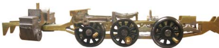
Above: Right: Making it all fit: test fitting the revised cylinders and smokebox saddle unit. Below: Body taking shape: boiler, tank and cab adjusted for length and height, ready for test fit on chassis.
