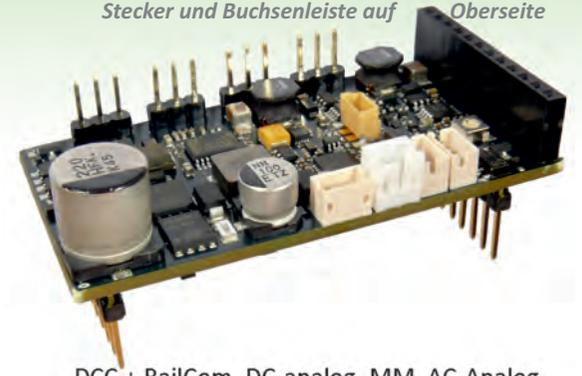
DCC + RailCom, DC-analog, MM, AC-Analog
