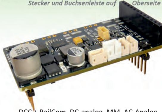
DCC + RailCom, DC-analog, MM, AC-Analog
