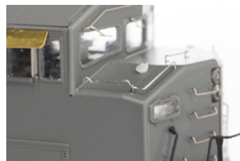
UP style tapered nose bevel with small sand fill hatches
