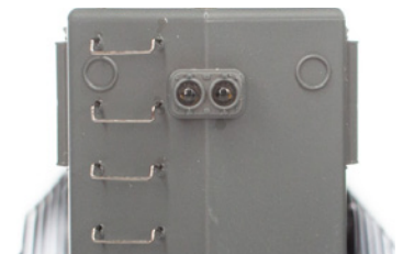
Late style rear high hood without rear numberboards and high gaskets
