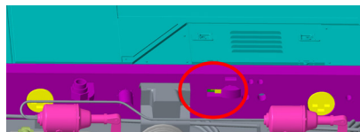
Illuminated ground lights
