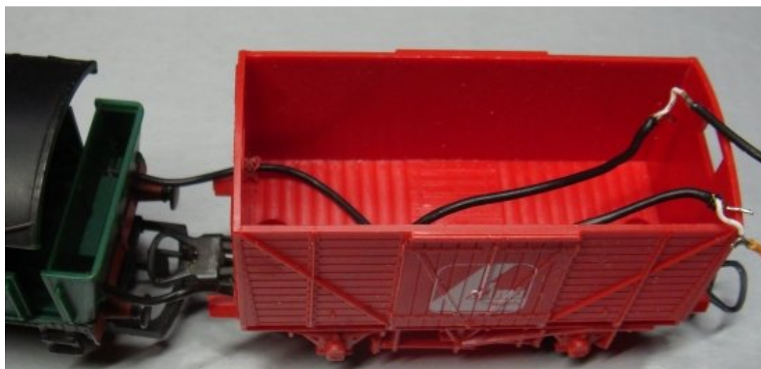
The Decoder can be put into a Coal Tender
