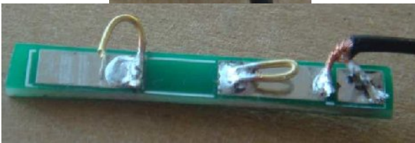
A close-up of the springy gold wires and the fine screened lead
