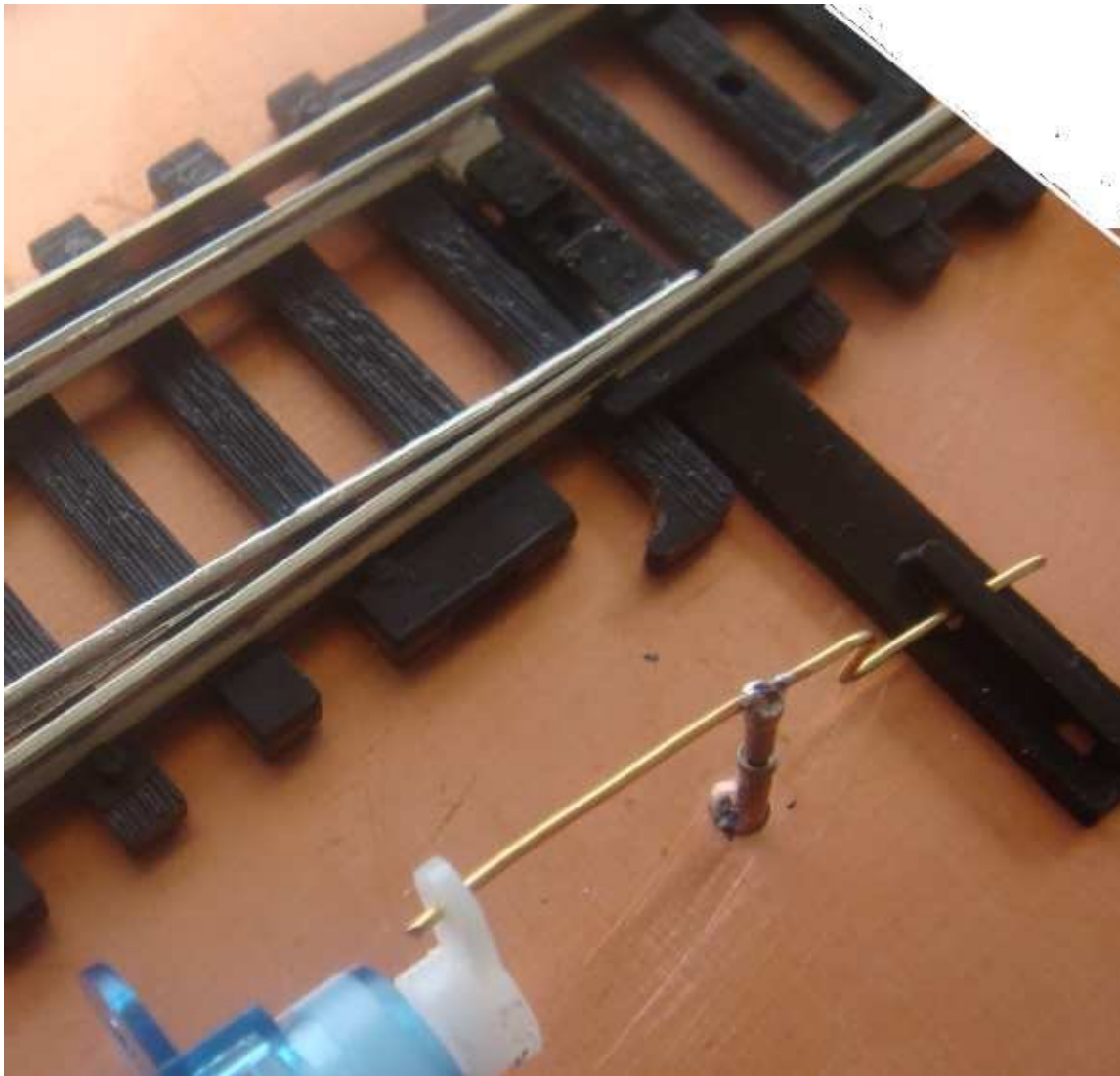
The Machine pin in the centre of the linkage acts as a pivot and the "crank" in the lever is simply to align the activating arm to the slider on the track. The gold wire is soldered to the pin so it does not change alignment.
