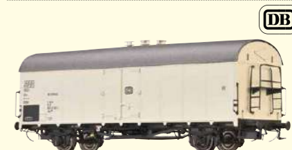
Kühlwagen Ibs 394 "INTERFRIGO" der DB Refrigerator Car Ibs 394 "INTERFRIGO" DB
