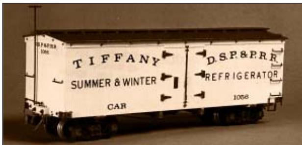
#29405 - DSP&P Tiffany Refrigerator Car The Tiffany Summer and Winter Car was one of the first cars built especially for refrigeration.
