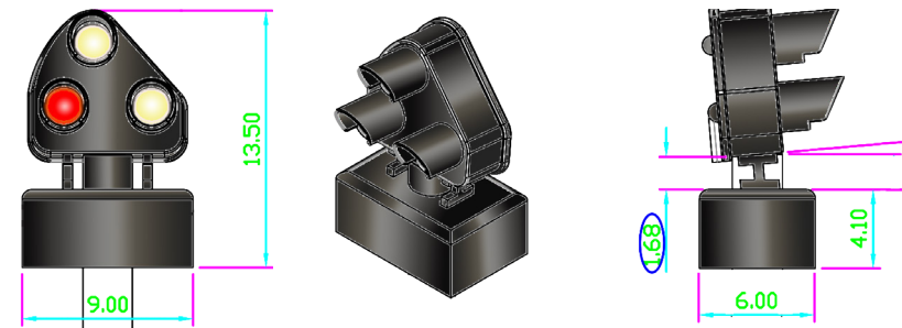
DCD-MGS-MG MODERN LED 4-LIGHT. SUCCESSOR TO THE 3-LIGHT SIGNAL.
