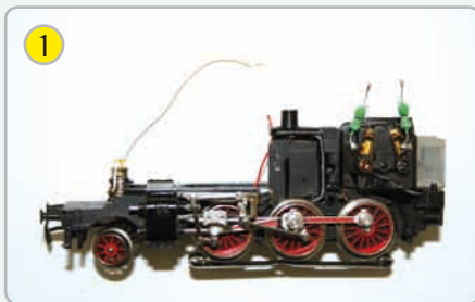
1 After adding the permanent magnet to the motor of your Delta® loco (as shown on the left page), remove the old Delta® decoder.
