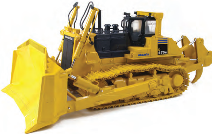
50-3230 Komatsu D475A-5EO Dozer with Ripper
