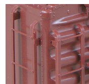
Scale ladders and grab irons.
