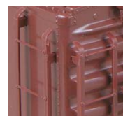
Scale ladders and grab irons.
