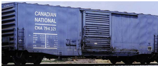
#6404 CNA #794321 .....$39.95 50' Boxcar - 10' Door, Built 1970, Repaint 2-86, Blue (Cushion Underframe)
