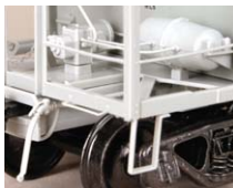
Scale rivets, grabs, air lines, chains, & AB valve
