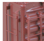
Scale ladders and grab irons.
