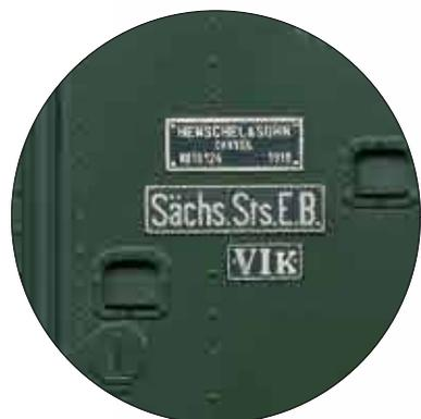
Locomotive builder plates separately applied as etched metal parts
