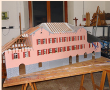
The shutters on the model's 84 windows are made of 4-millimeter thick PVC.
