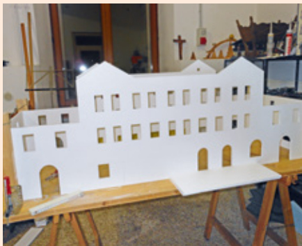
The large station building consists of 10-millimeter thick PVC boards.
