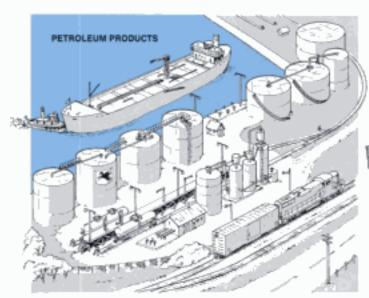
Petroleum products also keep the trains moving. There's a constant, though somewhat seasonal, demand for gasoline, fuel oil, heating oil, and kerosene products. Shipped in bulk by water, they are stored and blended in the tank farm at Free Haven, then distributed inland by tank car. The loading tracks can accommodate six cars at a time.
