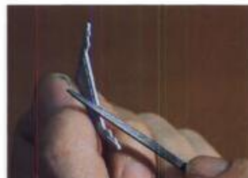
Fig. 4 NEEDLE FILES. Cleaning off the parting line makes this wood timber look more realistic.
