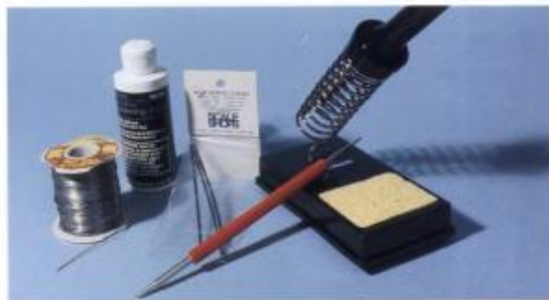
Fig. 1 SOLDERING SUPPLIES. A soldering stand safely holds the hot iron; this one also has a sponge to keep the tip clean. Liquid rosin flux and .025"-diameter rosin-core solder are excellent choices for model work. Heat-shrink tubing makes neater and smaller joints than electrical tape.
