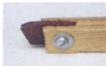
The Bright Boy abrasive track cleaner is an old standby that's still very useful. It can be mounted in a homemade handle to clean those hard-to-reach places.
