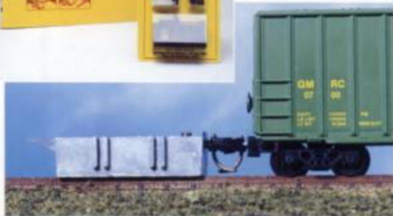
Fig. 4 ADJUSTING THE TRIP PIN. After your Micro-Trains couplers are mounted you'll need to make sure their height is correct using the Micro-Trains no. 1055 height gauge. The correct height for the trip pin is .010" above the railhead.
