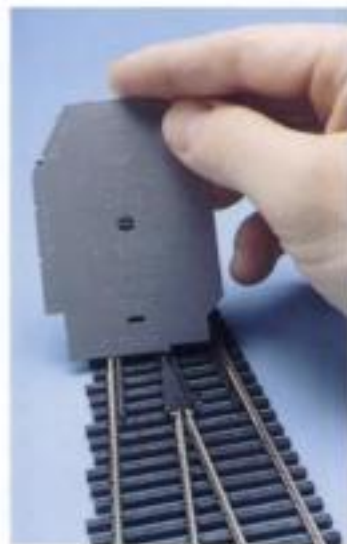
Fig. 5 NMRA GAUGE. These steel gauges allow modelers to easily check track components for conformance with the National Model Railroad Association's standards.
