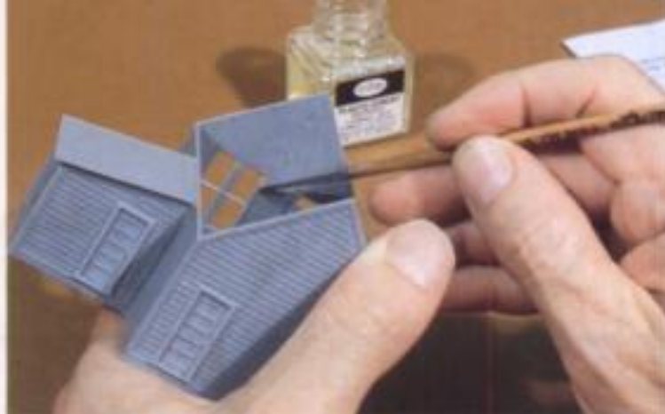
Apply liquid cement from the inside to avoid marring the plastic surfaces.
