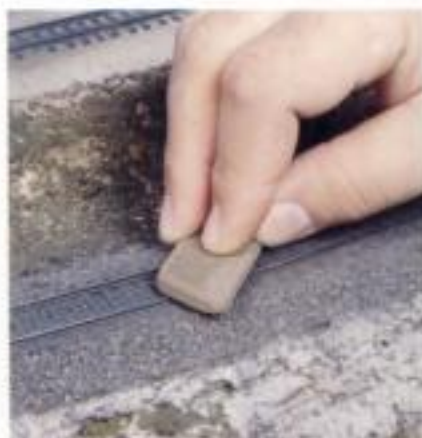
The Bright Boy abrasive track cleaner is an old standby that's still very useful. It can be mounted in a homemade handle to clean those hard-to-reach places.
