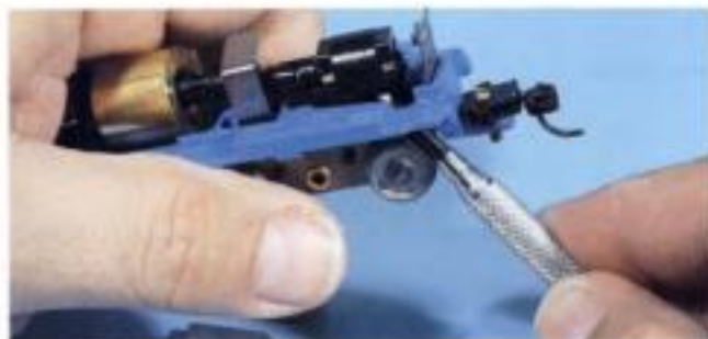
Fig. 2 REMOVING WORM HOUSING. Use a small screwdriver to gently pry off the combination worm housing and truck retainer.
