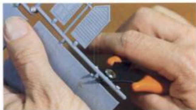
Fig. 2 REMOVING PARTS. Put the flush side of the cutter against the part and squeeze gently. Be sure and cut each sprue feeding the part.
