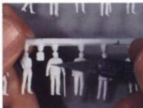
Fig. 2 CLEANING FLASH. Use a sharp knife to clean any flash from the back and extremities.
