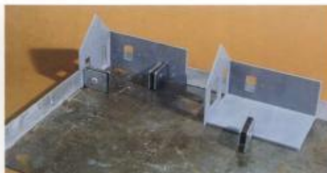
Fig. 5 SQUARE TABLE. A square table keeps corners square until the cement dries. Micro-Mark sells a similar unit as a "magnetic gluing jig."
