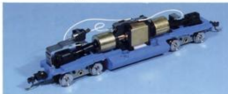
Fig. 7 NEW WIRING. Replace the original Athearn steel contact strap with flexible wires soldered in place to provide a more reliable electrical path.
