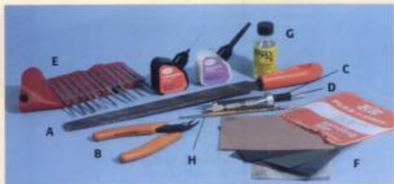
Fig. 1 BASIC TOOL KIT. A. 6-inch mill file for cleaning up sprue marks and parting lines. Buy a new one. B. Sprue cutters are flush-cutting pliers sold by many manufacturers. Don't use them for anything else. C. Hobby knives for clean up and removing parts. D. Needle files for removing flash, parting lines, and sprue marks. E. A pin vise holds small drills for hand drilling. If you're adding detail parts or changing coupler types you'll want one. F. Fine sandpaper, 440 grit and higher. G. Liquid styrene cement produces clean joints and sets quickly. Also pictured is Testor's clear cement for glazing windows. H. Fine brush for applying liquid cement.
