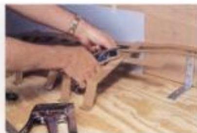
We used a pliers-type stapler to fasten the strips where they crossed. The angle iron seen on the right is matched by one on the opposite side of the backdrop and holds the backdrop in position.
