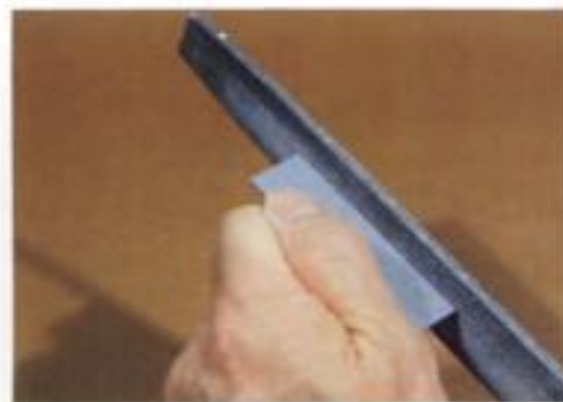
Fig. 3 MILL FILE. A large file keeps edges straight for strong glue joints and good looks.
