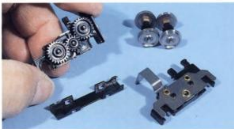
Fig. 4 GEARBOX. Clean off any molding flash or dirt found in the gearbox.
