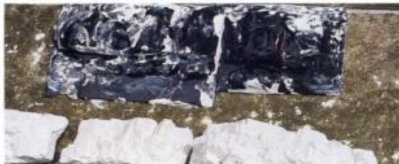
These two molds were applied to the slope while the plaster was still wet. The molds weren't removed until the plaster had thoroughly set.
