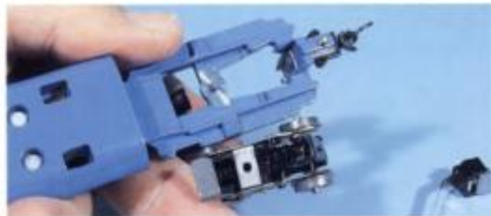
Fig. 3 TRUCK KINGPIN. Polish all electrical contact points where current is transferred between mechanical components.
