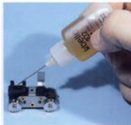
Fig. 6 LUBRICATION. Apply only a couple of drops of plastic-compatible lubrication in each truck gearbox.
