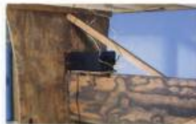
Fig. 9 WIRING. Jeff Wilson built this simple plywood shelf under the layout to support the power pack. The walk-around throttles plug into telephone jacks on the side of the layout.
