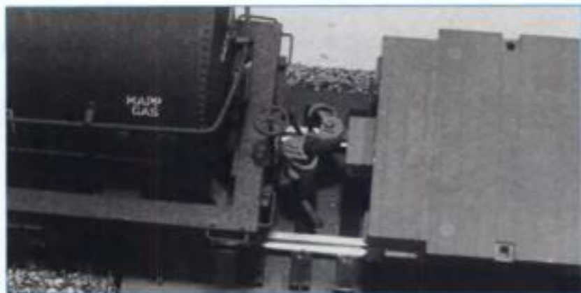
Fig. 1 DELAYED COUPLERS. Bringing Magne-Matic couplers together over an uncoupler shifts them off center so a car may be pushed and left at any spot beyond the magnet.
