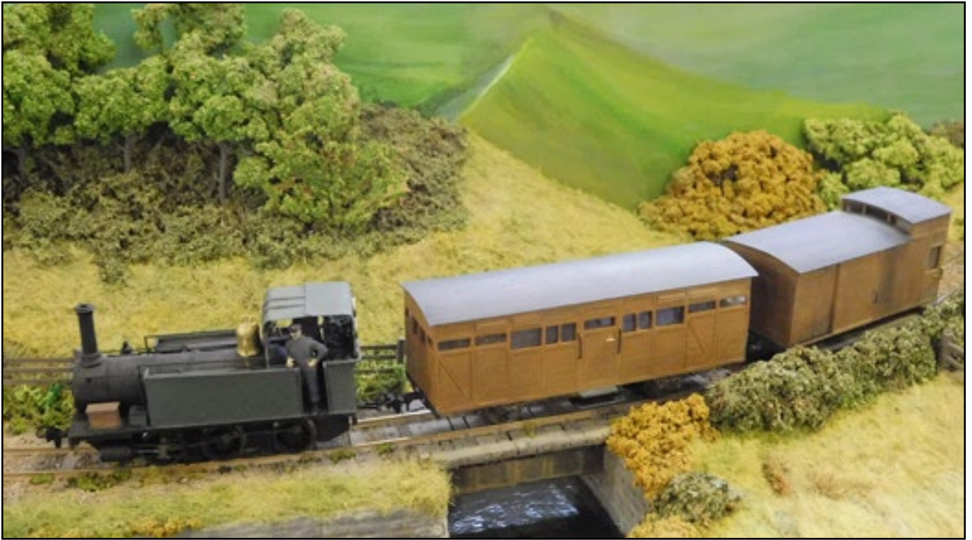
Original Ravenglass & Eskdale loco and train. Loco is built on Jouef/ Electrotren 0-6-0 chassis (David Hennessy).
