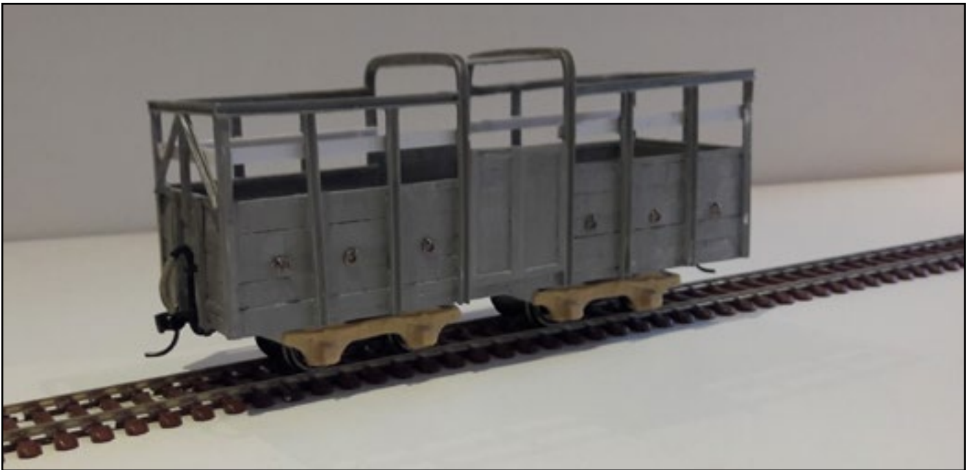
CGR 20' Cattle Wagon - scratch built and still under construction
