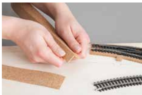
First the Cork Trackbed is bent in the middle ...
