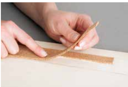
and the two strips are then glued with »the back side« against each other. Thus the Cork Trackbeds can be flexibly adapted to every route.
