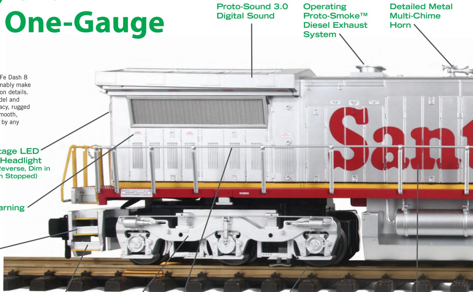
Constant Voltage LED Rule 17 Rear Headlight (Full Brightness in Reverse, Dim in Forward or When Stopped)
