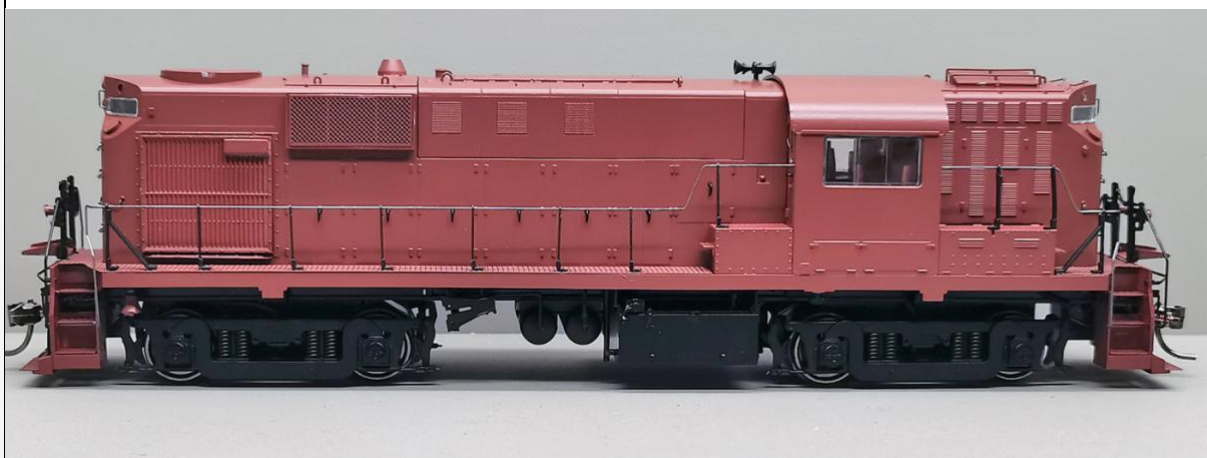
Note those short-hood dynamic brakes that were unique to DWP and CV. First pre-production sample shown.
