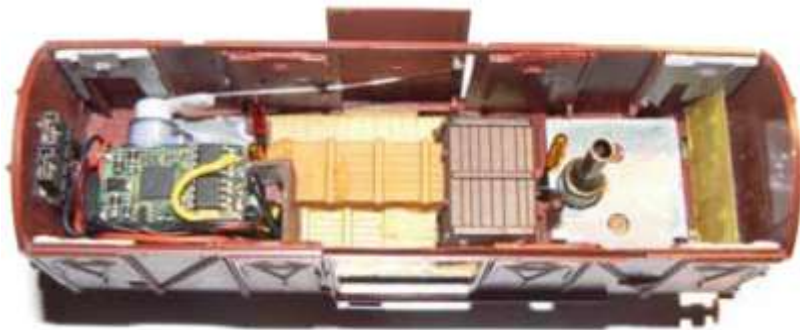
Application example: H0 Goods wagon with Digital Servo which opens the wagon door and Digital decoder for light and smoke
