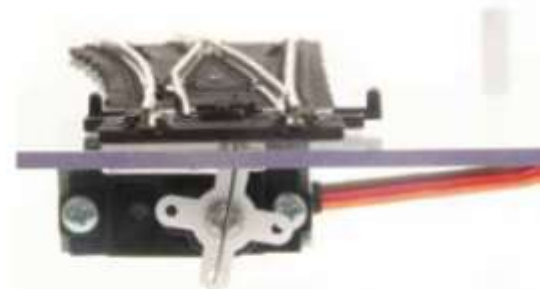
Application Example: The precision servo operates a turnout
