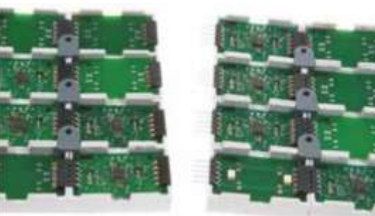
This is how a complete wired Uhlenbrock control panel looks from underneath.
