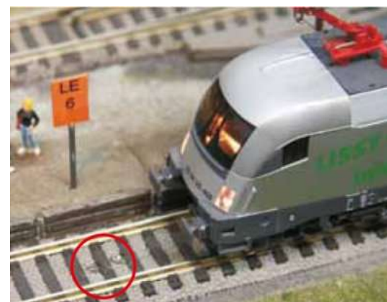
Barely visible: LISSY receiver sensors installed in the track
