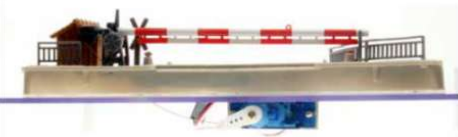
Application Example: The standard servo operates a boom gate
