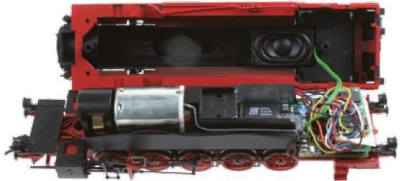
Example: Decoder 76 425, Sound module 32 300 and loudspeaker 31 110 installed in a PIKO BR94.
