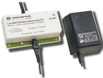
If the total power requirement of the attached LocoNet devices is larger than the maximum output current of the center a LocoNet Power feed unit is required. The power feed unit puts a further 500mA at the disposal of the LocoNet.
