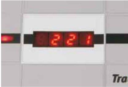
With installation of the individual locomotive control system »LISSY« or the modular automatic for RailCom »MARCo« the train numbers of the trains passing the designated LISSY sensor or the MARCo system track section are displayed, (e.g. at the exit track of the Shadow station).
