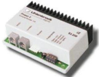
The Power 2 can be used as an additional booster in a digital system, which is controlled by an Intellibox or TwinCenter.
