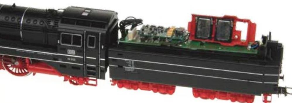
Sound decoder 35 330 and two 31 101 Loudspeakers installed in a Roco BR 10
