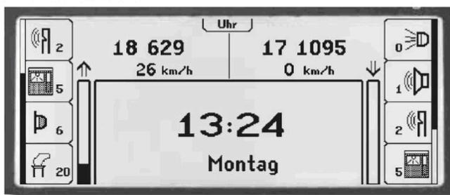
A prerequisite for timetable operation is a model time clock. The Intellibox II has a model time which can be incorporated in the display. It shows the time and the week day. This model time can run at normal time or accelerated by a factor between 1 and 127. The clock in the Intellibox II can also be synchronized with other clocks connected to the LocoNet.
