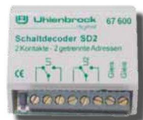
A universal switching decoder with two separated, two-way potential free contacts, addressed by two independent addresses. The decoder independently switches two different items, for example lamps or a motor, to operate a turnout.
