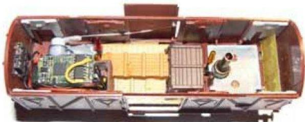
*HO Goods wagon with a digital servo that opens a wagon door and digital decoder for light and smoke.*
