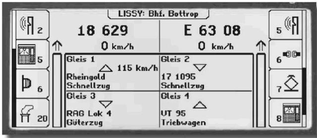
In automatic operations just like with manual control you always have the question: "Which Locomotive is at which location on the layout at any particular time?" With LISSY or MARCO the Intellibox II can easily answer this question. In LISSY Mode it provides the following Information:
