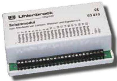
Our LocoNet Switch Module is a clever device. A single module which can achieve all switching processes on your layout. The Switch Module can switch lighting, turnouts, uncoupling tracks, semaphore signals, light signals, level crossings and effect lighting. All these switching tasks can be mixed with a single Module.
