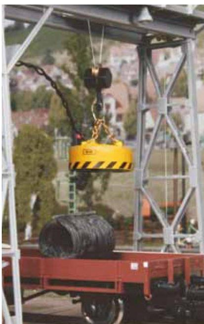
Model of Load lifting magnet BvM L34-170 from the J. Braun GmbH. Company.
