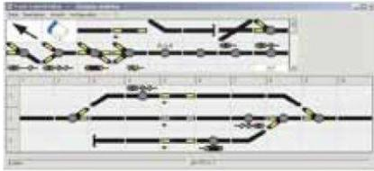
1. Plan your control panel with the provided planning software on the PC. Print the track plan, the connecting plan and the parts list.
