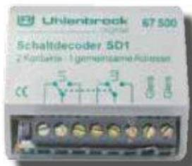
Universal switching decoder has two separated two-way potential free contacts, which are addressed by one address. One contact can, for example, switch a light signal and the second, the track power.
