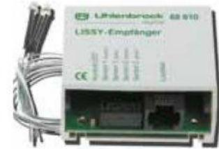
In places where a travel direction dependent automatic function is to be implemented, the two sensors of a receiver are installed in the track one behind the other. In addition to the address and train category the speed and travel direction can be determined.
