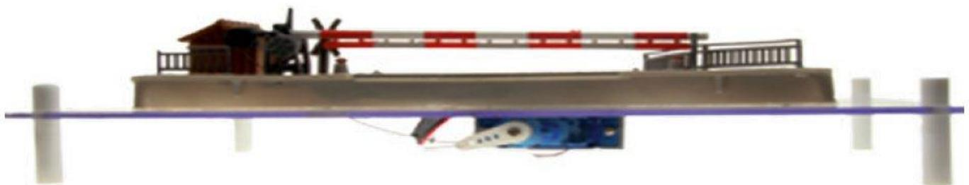
The Standard Servo operates a boom gate.
