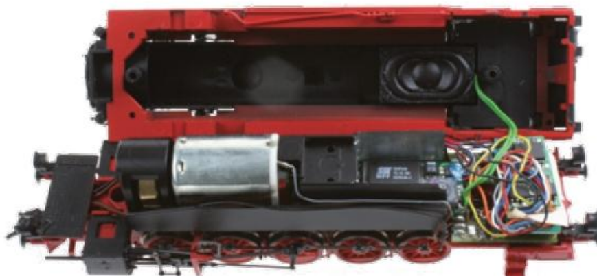
Example: Decoder 76 425, Sound module 32 300 and loudspeaker 31 110 installed in a PIKO BR94
