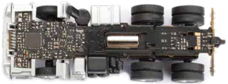
The circuit board serves as chassis.
