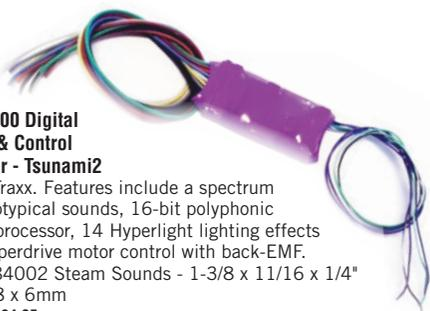
**TSU-2200 Digital Sound & Control Decoder - Tsunami2**
