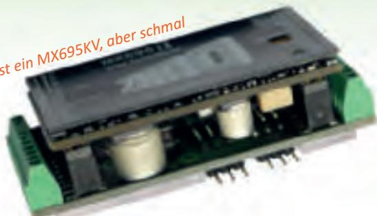
DCC + RailCom, DC-analog, MM, AC-Analog
