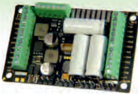
DCC + RailCom, DC-analog, MM, AC-Analog
