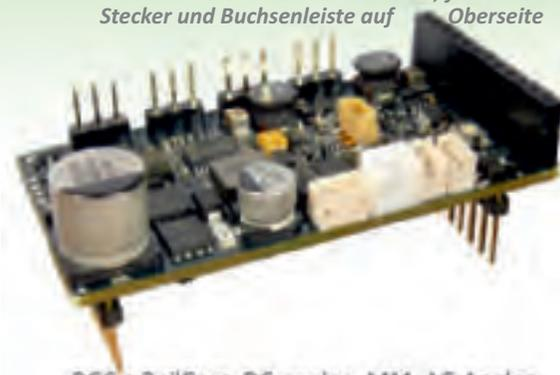
DCC + RailCom, DC-analog, MM, AC-Analog
