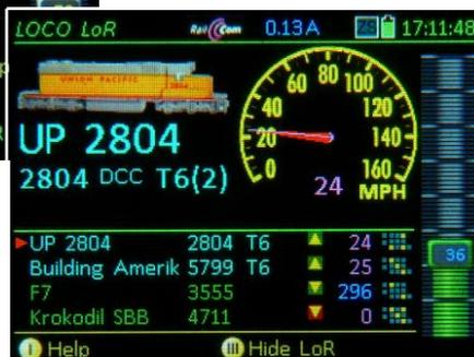
Example on the left (image 1): Locomotive „UP 2804“ was brought to the foreground (from the **LoR**, the **ObjDB** or input of the address). This loco is part of a consist on another cab, thus marked „FT(2)“ (external consist with two locos).
