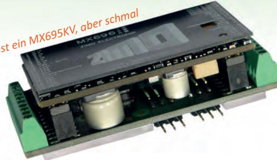
DCC + RailCom, DC-analog, MM, AC-Analog
