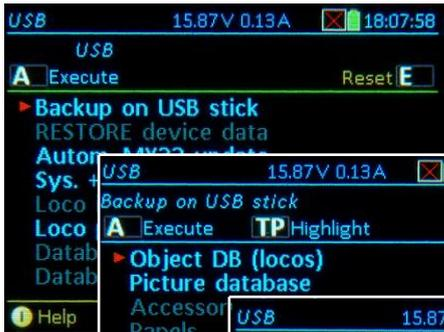
A lot of work is mostly put in the content (i.e. **Object Database**, pictures, panels etc... of the cab MX32) created by the user himself. A newly available **backup** now ensures, that this work is safe for use in other MX32's or in case of damage. A **reloading of the data** is possible either complementary or by replacing the original data.
